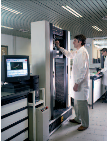
Offset Printing Blankets compressibility test. Photo Trelleborg.
