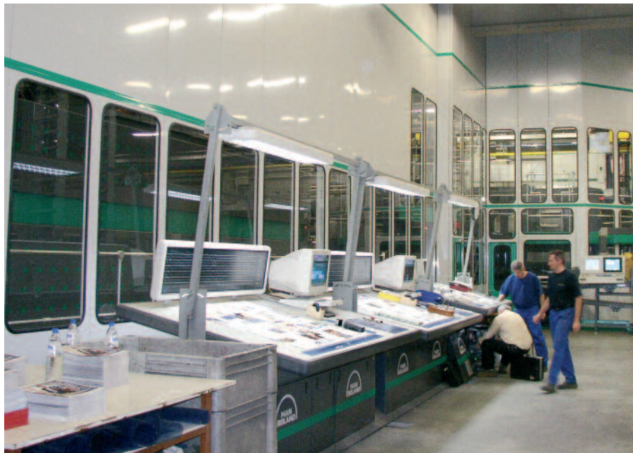
Correctly installed hermetic soundproofing reduces noise level below 80 dB(A) to not only ensure employees' health but also helps minimise energy loss. Source Faist.
