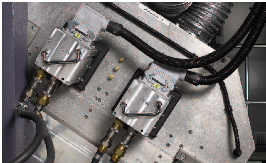
A Blanket-to-blanket press UV installation. B Satellite press UV installation between the upper and lower satellites. Source manroland.
