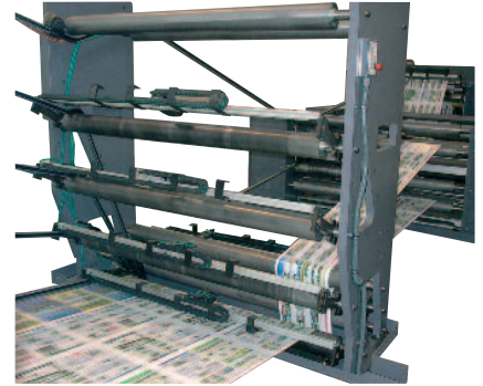
The photograph shows the UNISSET heatset web leaving the MEGTEC dryer (in the background to the right). The web is then split into two, and one half becomes the newspaper's 4-page cover that is merged with the coldset double-width web in the REGIOMAN folder superstructure (foreground). Photo: DIC Australia.
