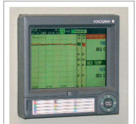
Chart recorder monitors oxidiser combustion chamber temperature to indicate CO and VOC destruction.
